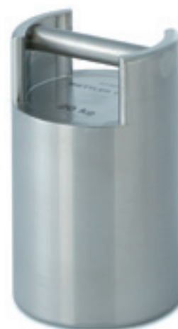
Calibration weights must be certified and traceable
